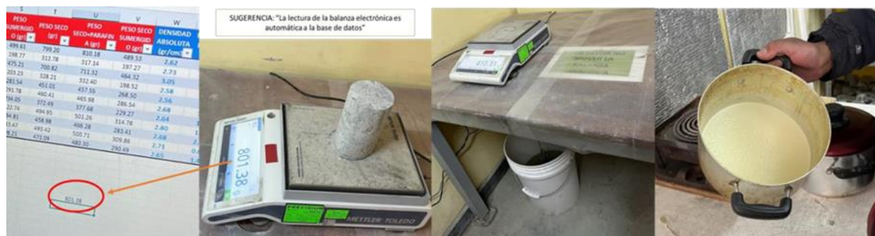
Figure 11-12 Determination of bulk density (diamond drill core example) by the water immersion method
