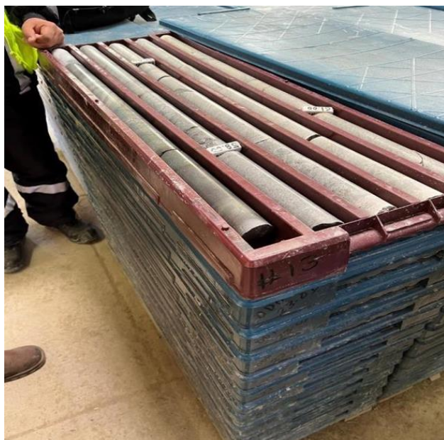
Figure 11-3 Correctly aligned core for measurement of core recovery and RQD
