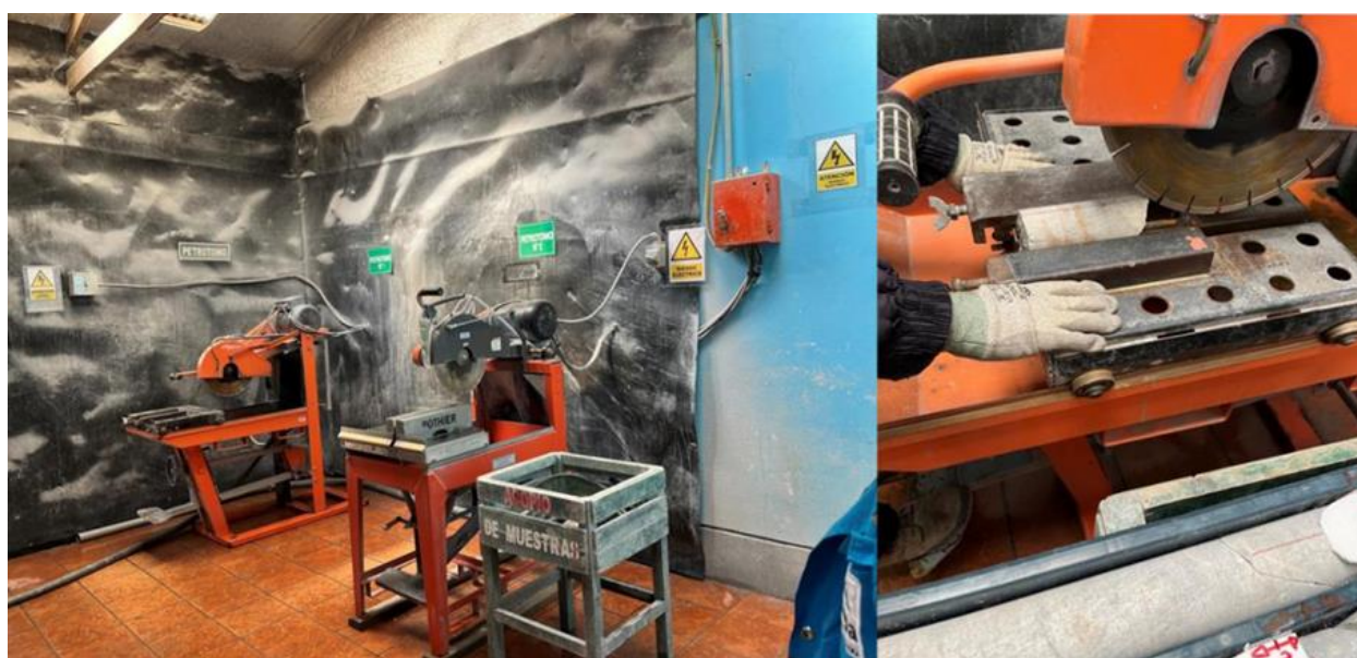
Figure 11-6 Kolpa symmetrical splitting of mineralized core in preparation for sampling and analytical analysis
