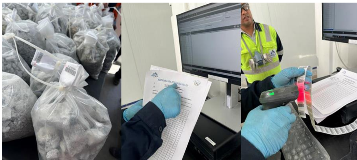
Figure 11-8 Receipt of samples and capture into the LIMS system at the Kolpa mine-site analytical laboratory
