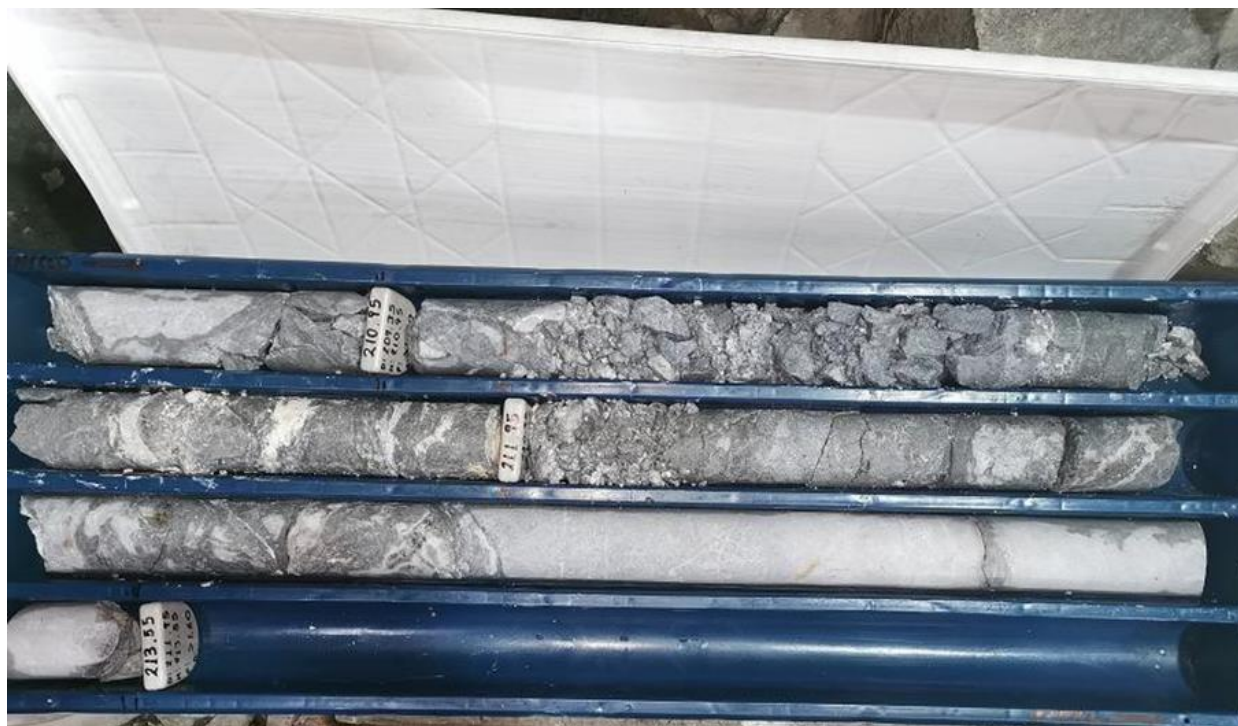
Figure 11-1 Plastic core-holder box with strong lid and depth marker blocks
