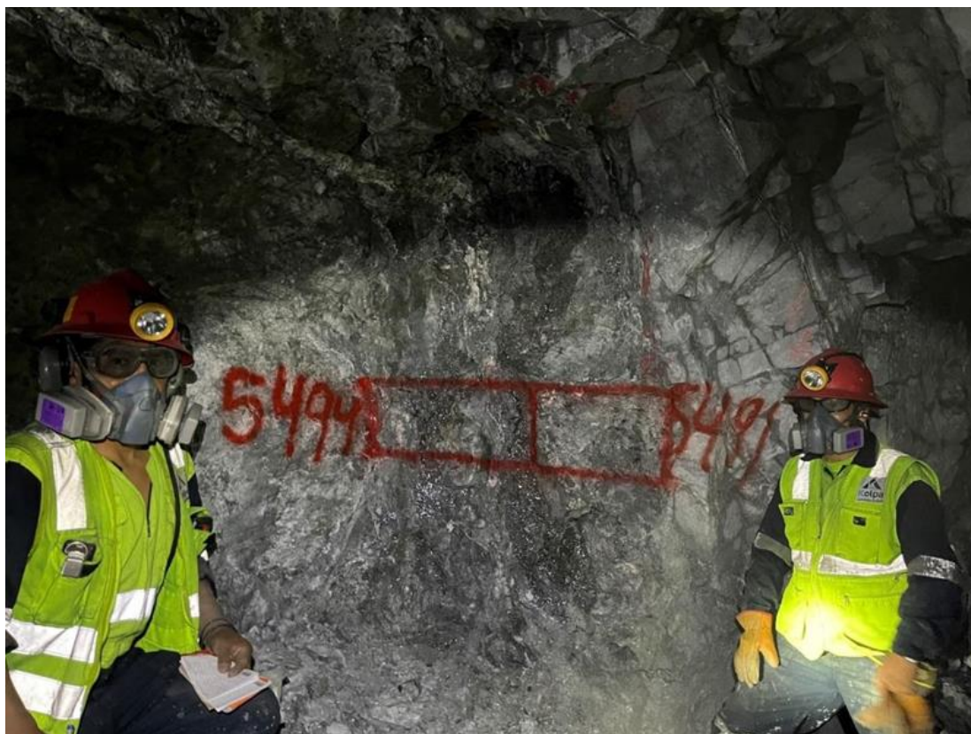
Figure 11-9 Marked-out sub-horizontal channel sample on a sub-vertically oriented polymetallic vein
