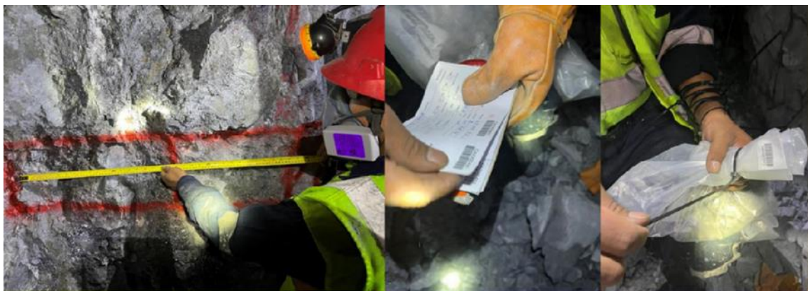
Figure 11-11 Measuring limits of a sub-horizontal channel sample; coded sample tags and sealing of sample bag
