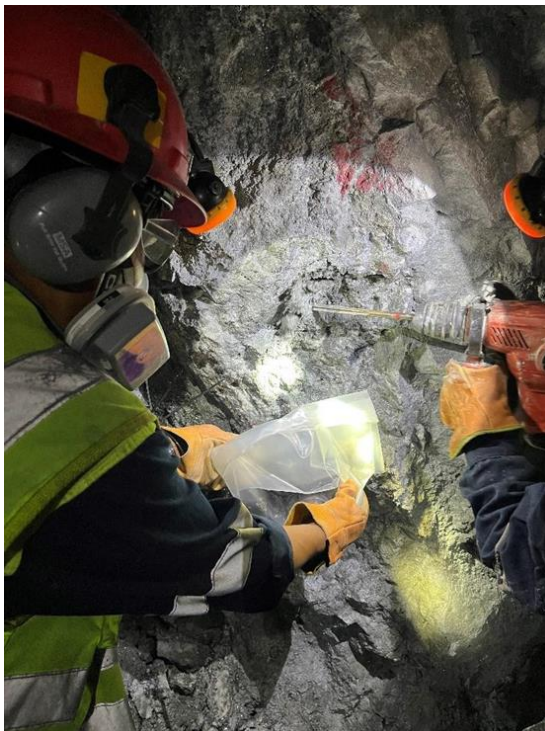
Figure 11-10 Collection of a channel sample from the mineralized structure directly into a plastic sample bag
