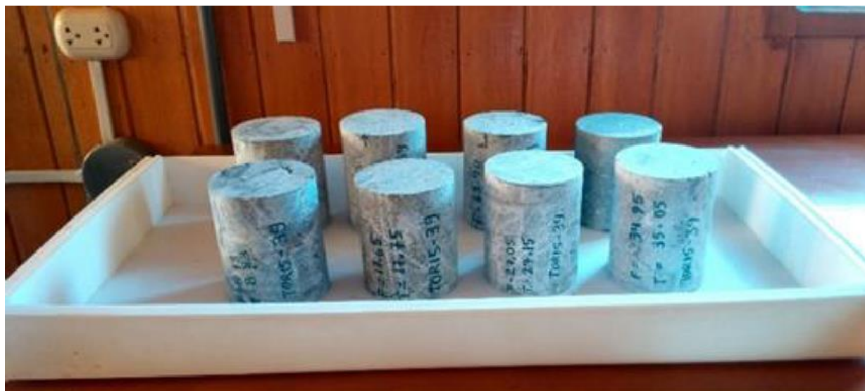
Figure 11-13 Carefully and clearly labelled 10 cm long HQ-diameter drill core bulk density samples
